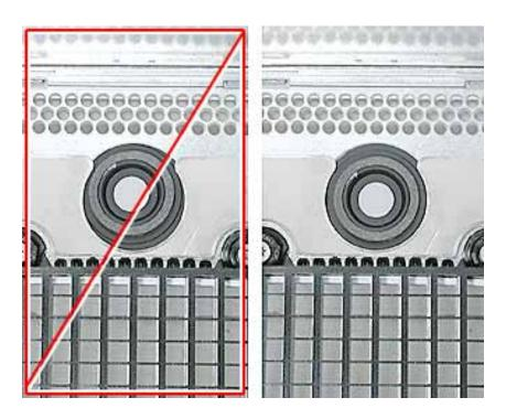
2 Holding the core by the latch, insert the core into the enclosure. (Figure 20)
